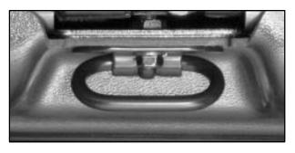
There are two cargo tie downs located on the inside of the liftgate in the rear of the vehicle to secure cargo inside the vehicle with the liftgate closed.
